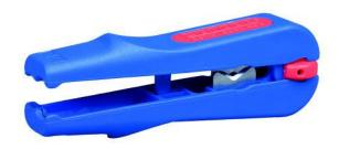
The Combi-Coax No. 3 allows two- or three-level stripping of all common coaxial cables, NYM cables and flexible cables. There is no need to adjust the cutting depth. The Combi-Coax No. 3 strips coaxial cables with a diameter of 4.8-7.5~mm, NYM cables of  $3 \times 0.75~\text{mm}^2$  and flexible cables of 10 and 16 mm².
